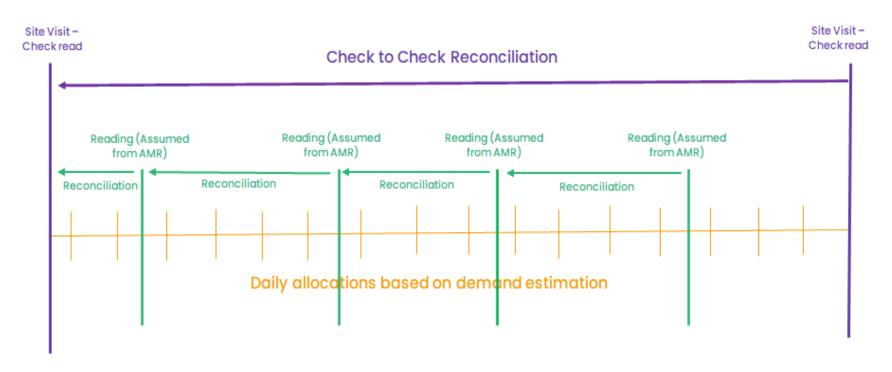
The Check to Check reconciliation apportions any 'drift' between the meter & the AMR to the previous Check Read
