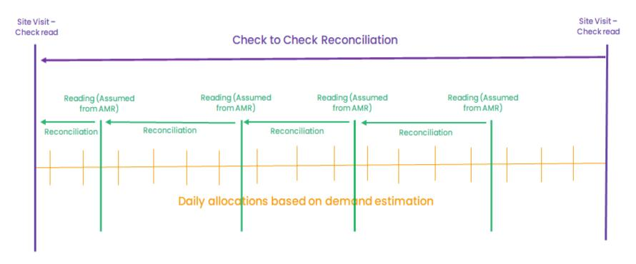
The Check to Check reconciliation apportions any 'drift' between the meter & the AMR to the previous Check Read
