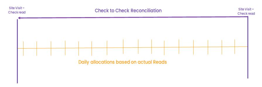
The Check to Check reconciliation apportions any 'drift' between the meter & the AMR to the previous Check Read
